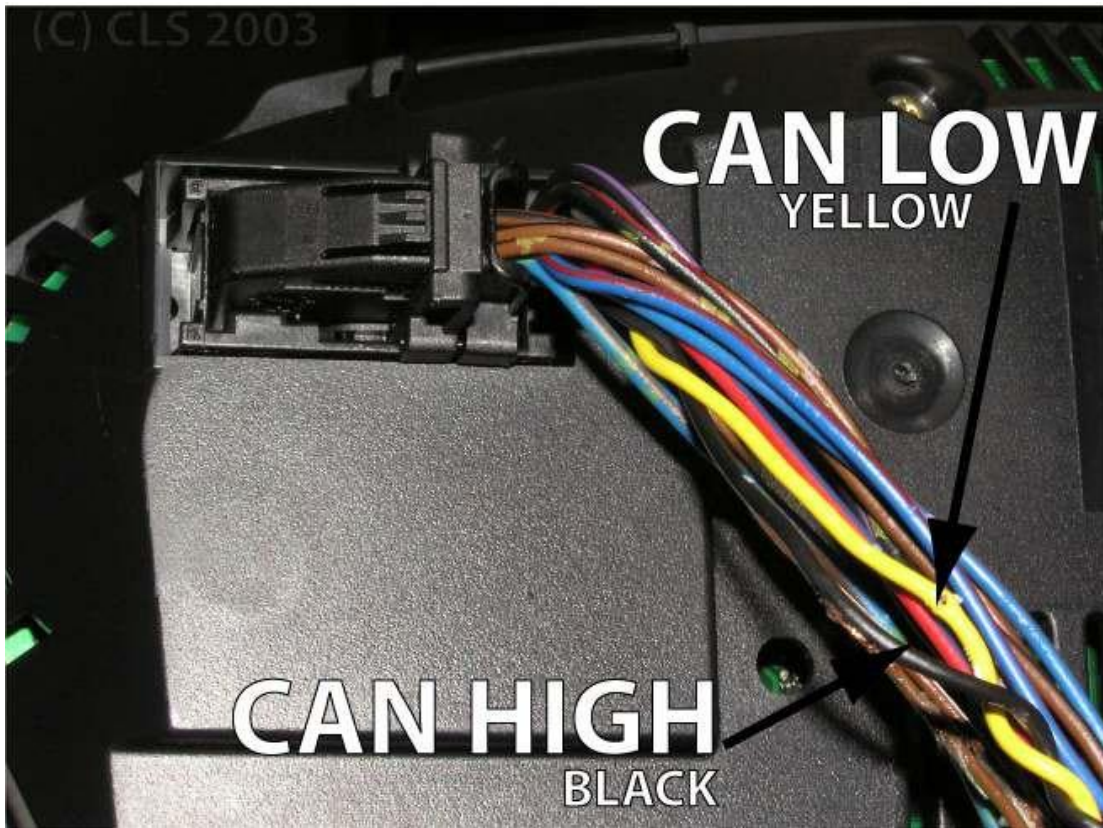
Picture from 2003 Model BMW 53 series Wiring on rear of instrument cluster
